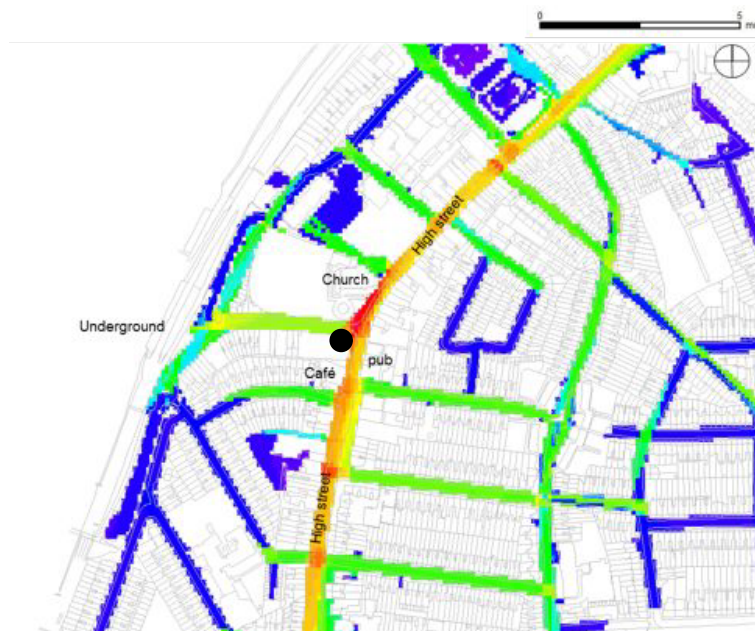
Fig.n. 2 – Spatial configuration of Leytonstone. The figure shows visual integration, which explains occupational potentials for space and the likelihood for people to stand or interact. The visual integration goes from high marked in red to low marked with blue. The display location is indicated with a black dot.
